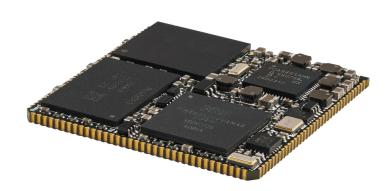
UCM-iMX95 is based on NXP's very latest iMX95 processor, providing high performance graphics and image processing and optimised for industrial applications.
